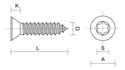
Countersunk screw lengths L are always measured including the head.
